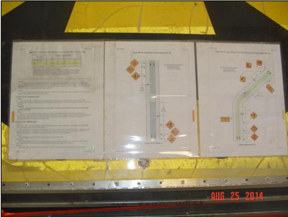
MUTCD sign layouts are attached to the inside cover with waterproof covering for quick reference.
